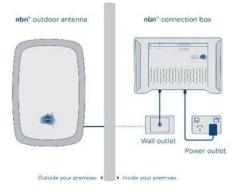
This is the most common technology for rural areas or whenever is not possible to use any other technology. An external antenna is connected with fibre optic to the NTD, which should be inside the premises, which looks like the image above.
